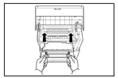
Insert the *Developer Unit* together with the *Toner Container*, back into the machine.
